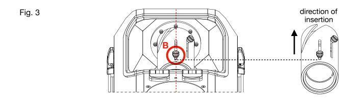
To take advantage of the maximum extension of the lens you need to place the knobs at the ends, as in Figure 3. Then place the image (Gobo or dynamic effect) centrally and flat on the plate, following the guides. The ideal focus can be found by moving the image back and forth, as shown in Fig. 4.
