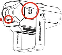
Insert the chosen lens into the projector by making sure that knob B is centered relative to the sagittal axis of the projector, see Fig. 3. Then attach it to the machine body by rotating the A element on the outside, see Fig. 2.
